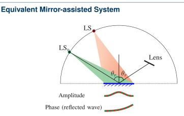
**Helpful result [R3]:** The IRS phase shift can be chosen such that the phase of the non-specular reflected wave from the IRS in the original system becomes identical to the phase of the (specular) reflected wave from a mirror in the equivalent system!
