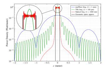
Power density of the reflected wave at *x* and y = 200 m. An IRS located at origin on the *x*-axis with size 20 cm anomalously reflects an oblique plane wave impinged from angle 30° into perpendicular direction [R1].
