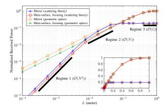
Fraction of transmit power received by an Rx lens vs. the IRS length *L*. Setup: 2D system; Tx at (-200 m, 300 m); IRS at (0,0), Rx at (0,500 m); Gaussian beam; 1550 nm wavelength; waist radius  $w_0 = 1 \text{ mm}$ ; IRS length *L*; half-wavelength unit-cell spacing; Rx lens length 10 cm [R1].
