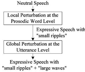
Fig. 4. Integrated local and global perturbation model for expressive speech synthesis.
