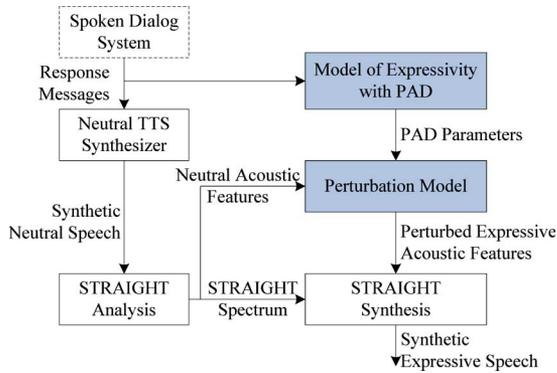
Fig. 1. Overview of the expressive text-to-speech (E-TTS) synthesizer for response generation in a spoken dialog system.
