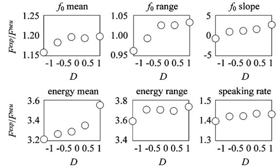
Fig. 3. Ratio between expressive and neutral speech acoustic features  $F^{\text{exp}}/F^{\text{neu}}$  for different  $D$  values.
