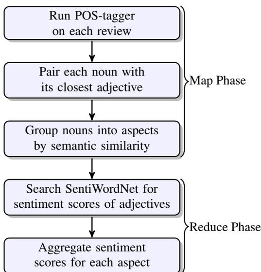
Figure 1: Block diagram of the Semantic-based Approach for Aspect-level Opinion Mining.
