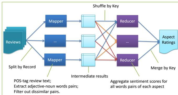
Figure 3: MapReduce Implementation for the Semantic-based Approach.
