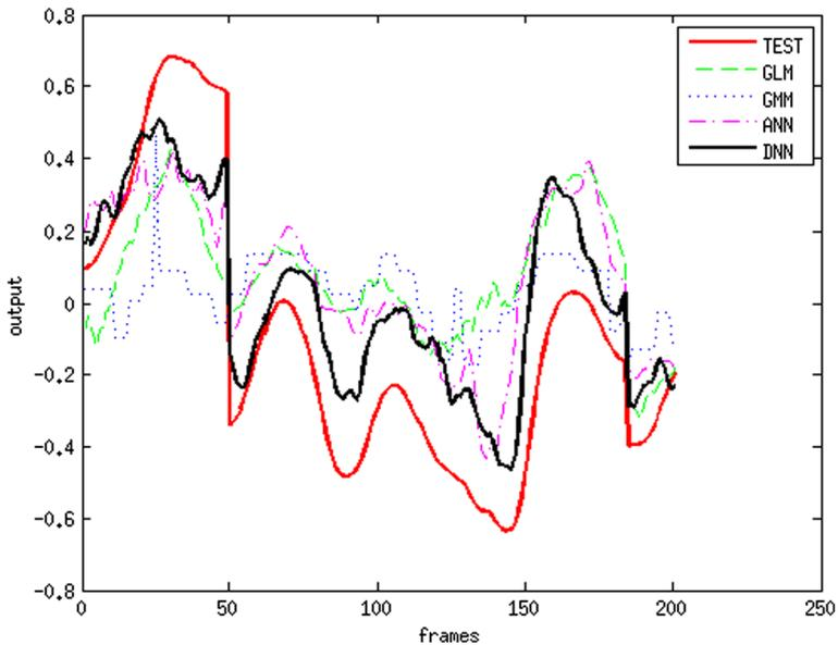
**Fig. 4** Comparison between the actually measured (red and bold curve, TEST) and the estimated articulatory trajectories for 200 frames of the tongue blade feature (T2) for GLM, GMM, ANN and DNN, where DNN (black and bold curve) achieves the best performance
