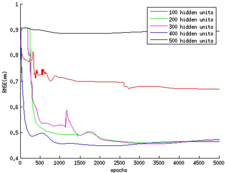
**Fig. 3** RMSE error of the estimated articulatory features as a function of epochs during DNN training on the validation set
