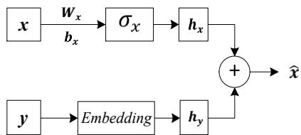
**Fig.1.** The structure of conditioned input layer.
