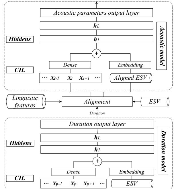
**Fig.2.** Schematic of proposed system,  $\{h_1, \dots, h_L\}$  presents BLSTM-RNN hidden layers,  $X_p$  and  $X_t$  are the phone-level and frame-aligned linguistic inputs.
