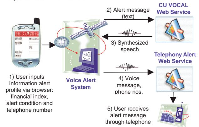
Figure 2. System architecture of the CU VOCAL voice alert system that integrates several Web services.
