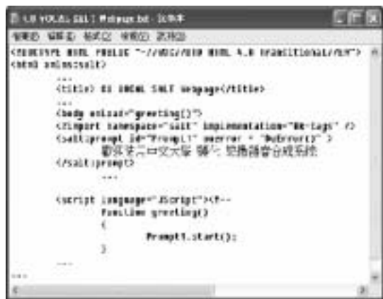
Figure 9. Underlying software implementation for Figure 8 illustrating how SALT tags were used.
