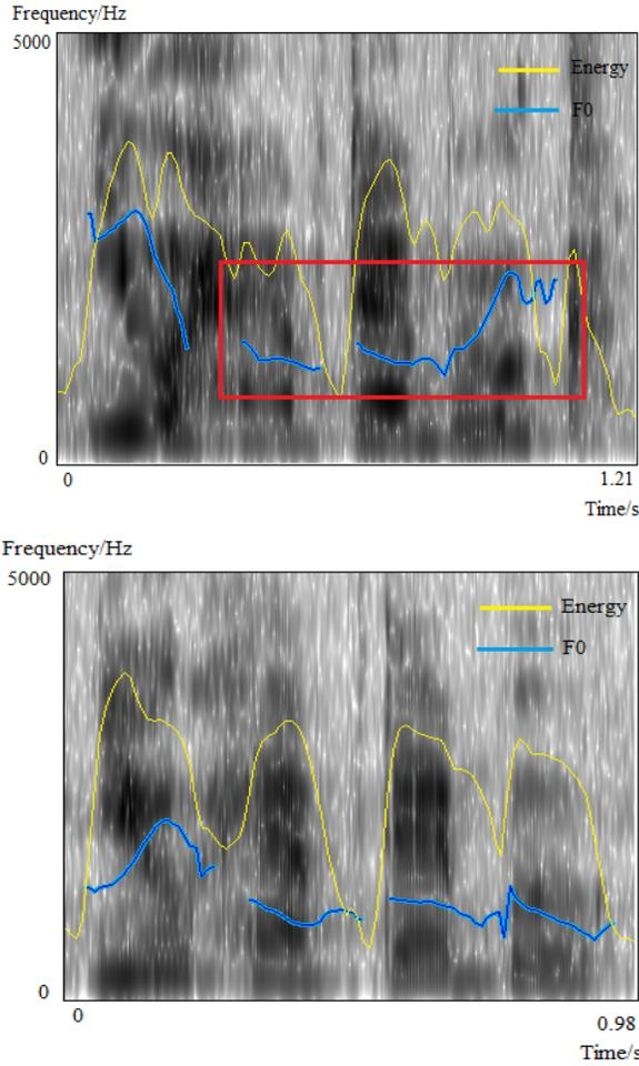
Fig. 1. The spectrum as well as the F0 and energy contours of the speech recordings with different intonations. Top figure comes from the speech with question intonation and bottom figure from the speech with neutral intonation. The blue curve is the F0 contour and the yellow curve is the energy contour. As can be seen, the F0 value in the red rectangle area increases gradually.
