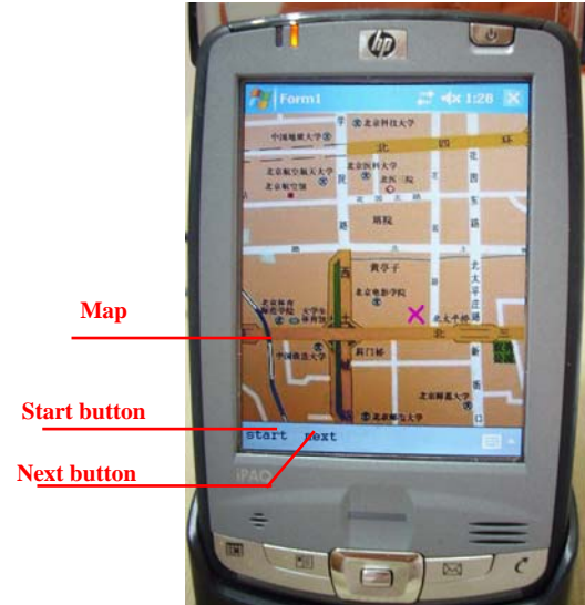
Figure 1. Data collection interface of the Pocket PC, augmented with soft buttons for logging functions (start/stop) and loading the next map.
