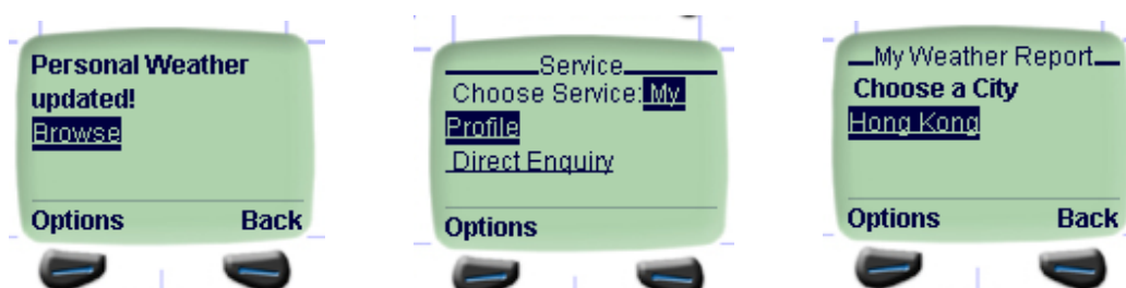
Figure 5. The weather information requested by the user in the spoken dialog interaction is ultimately pushed to his WAP phone as shown in the three screen dumps above.
