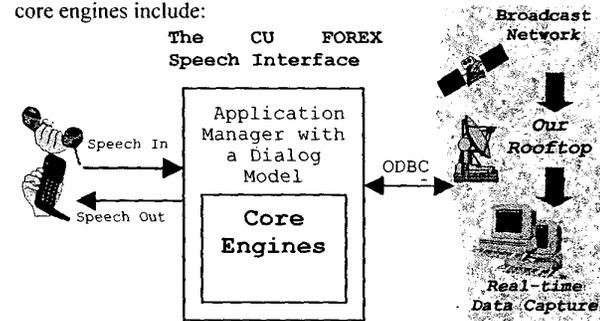
Figure 1: The CU FOREX System – overall architecture.
