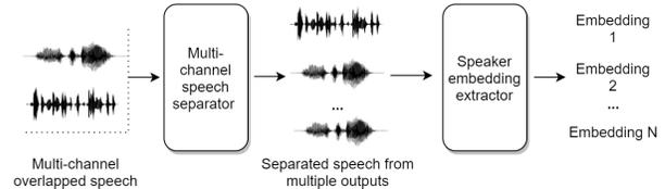
**Fig. 1.** The integrated system of the speech separator and the speaker embedding extractor.
