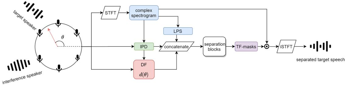
Fig. 2. Multi-channel speech separation network with look direction  $\theta$ .
