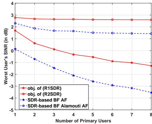
Fig. 7. Worst user's SINR versus number of primary users in the distributed CR relay network:  $L = 8$ ,  $G = 2$ ,  $M = 12$ ,  $\bar{P}_0 = 10\text{dB}$ ,  $\eta_u = 3\text{dB}$  for  $u = 1, \dots, U$ ,  $\sigma_{\text{ant}}^2 = \sigma_{\text{user}}^2 = 0.25$ ,  $\sigma_u^2 = 0.25$  for  $u = 1, \dots, U$ .
